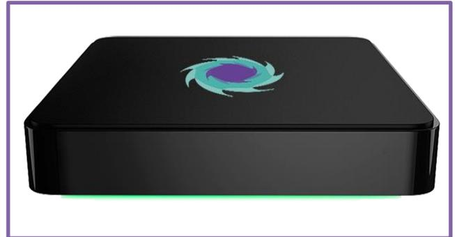
**BYOD Support for the Conference Room or Classroom.** Users can bring virtually any device into a meeting and share content to the Solstice wireless display. The Pod deploys client software to Windows and OSX computers automatically without the need for an external Internet connection or administrator privileges. For mobile devices, the Pod directs users to the correct app store download page for a free install of the client app (Internet access required for mobile devices).
