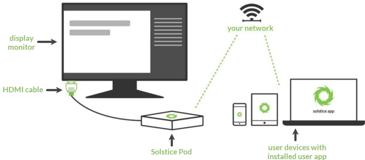
The requirements for an operational Solstice system are straightforward. The Solstice Pod is directly connected to a display monitor via HDMI cable. The Solstice Pod is then attached to the WiFi/Ethernet network that participants will use to connect and share to the display. Then, users on the network can follow the on-screen instructions to get the Solstice app and connect to the display.
