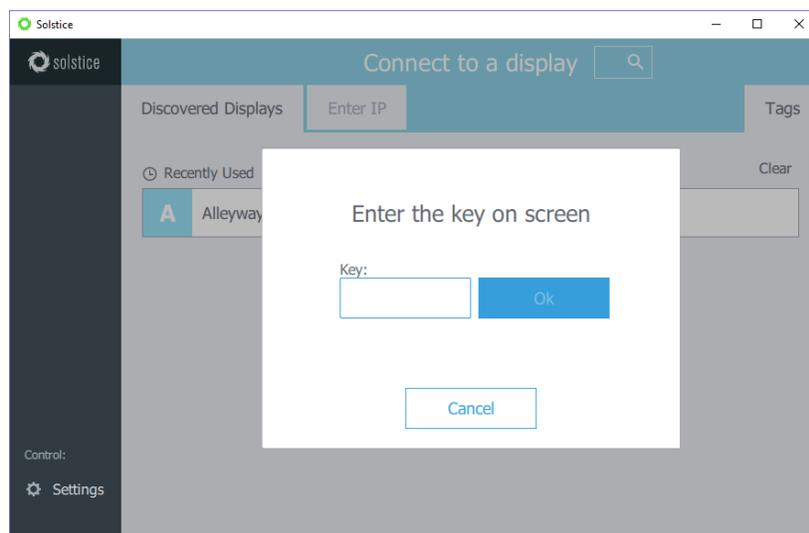
If you are unable to see any Pods to connect to, you can select the "Enter IP" option and type the IP address visible on the Solstice Pod welcome screen.
